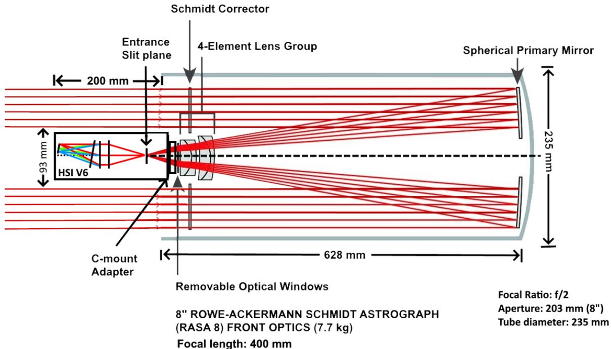
**Figure 2.** The 8" Celestron Rowe – Ackermann Schmidt Astrograph (RASA 8) as front optics to the HSI v6.
