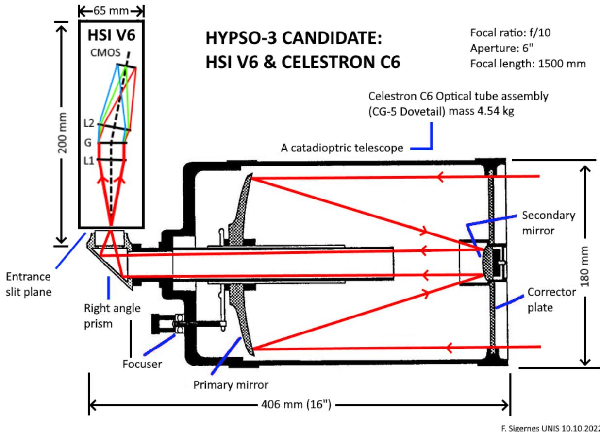
**Figure 1.** The 6" Celestron Schmidt-Cassegrain (C6) as front optics to the HSI v6. L1 collimator lens objective, G transmission grating, L2 camera lens objective and CMOS image sensor.
