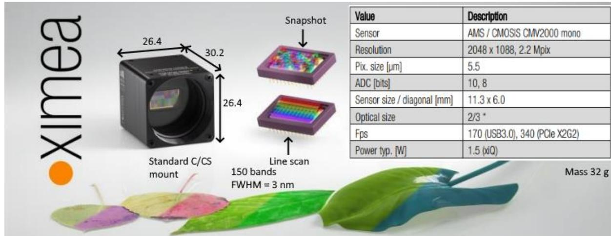
**Figure 2.** The 8" The XIMEA Hyper Spectral Imaging camera sensor with specifications. Dimensions are in mm.
